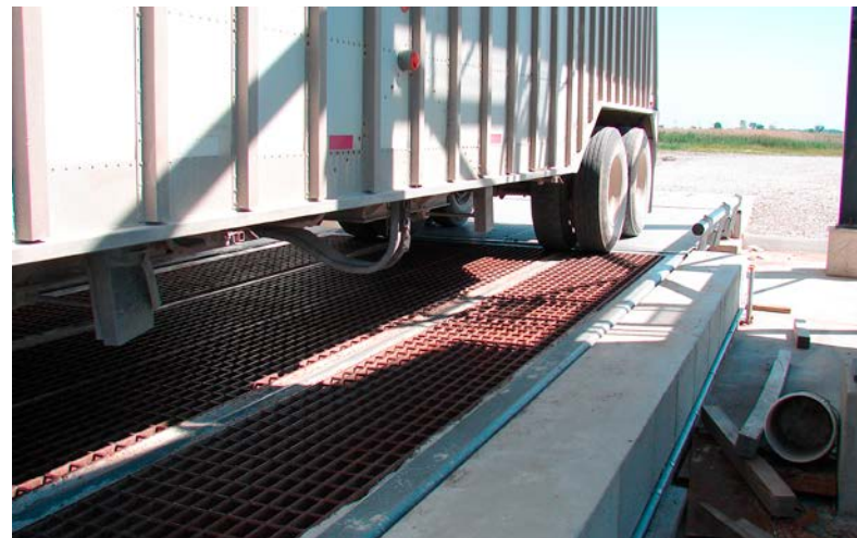
Processes are streamlined by integrating grain dumps directly into the weighbridge.
